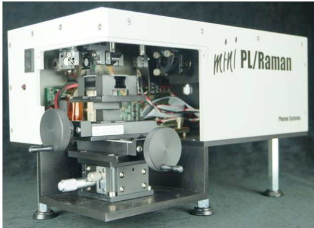
The Mini PL 110 standard configuration has a high precision manual stage
