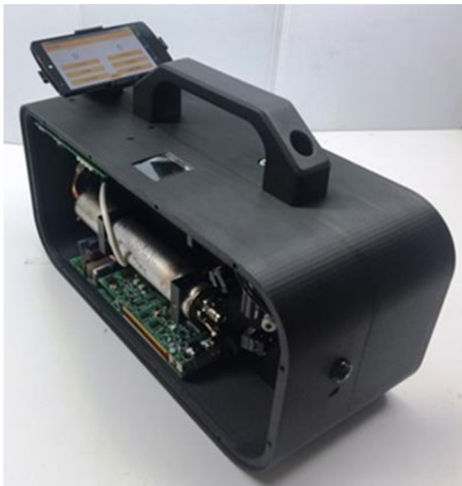
Figure 7. BRANE 1.0 deep UV native fluorescence sensor
