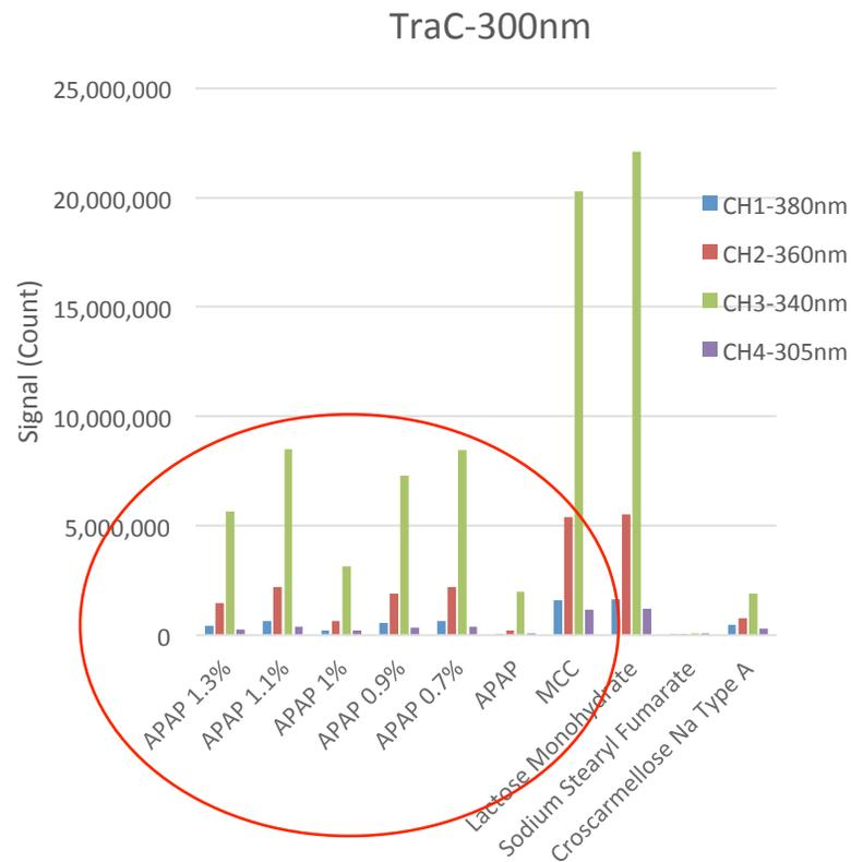
Looking at both versions of the TraC (300nm and 400nm) we see no concentration trend in the APAP dilution/concentration samples. Recalling the peak emission wavelength for APAP is ~325nm we would look at channel 4 on the TraC-400 device and at 340nm band(channel 3) on the TraC-300 instrument. You see on the TraC300 the Green (340nm) band is indeed highest but that is a result of the combined fluorescence of both the APAP and MCC with no way to differentiate the contribution of each.
