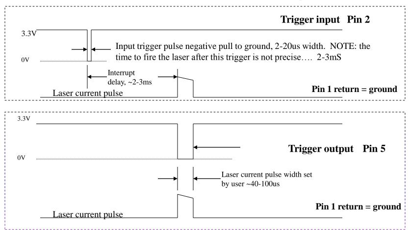
Trigger out occurs simultaneous with the input laser current pulse. Even if the laser is in Free Run mode this signal appears on Pin 5. It is best to trigger your experiment with this pulse if possible.
