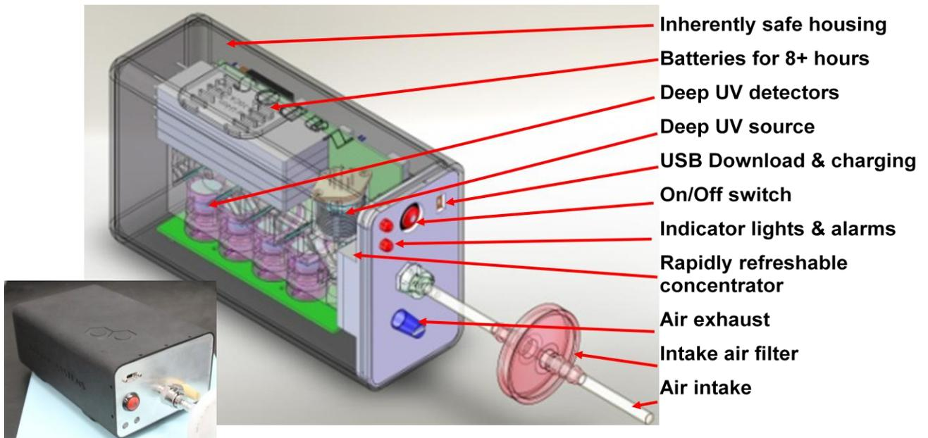
Figure 4. Illustration of VOCDoS sensor with key features along with a photo of Gen 3 version (inset)
