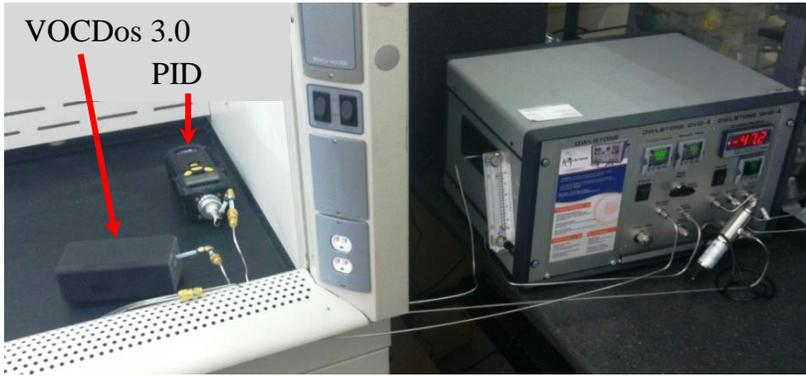
using a Owlstone OVG-4 vapor generator, which can generate NIST traceable, precise, repeatable and accurate concentrations of chemicals such as naphthalene. It can also co-mix with accurate generation of water vapor. A photo of our Owlstone generator next to a vent hood with a VOCDos 3.0 sensor and a Rae ppb PID (photoionization detector) is shown in Fig. 6. The range of capability of the Owlstone ranges from 1  $\mu\text{g}/\text{m}^3$  to about 6  $\text{mg}/\text{m}^3$ .
