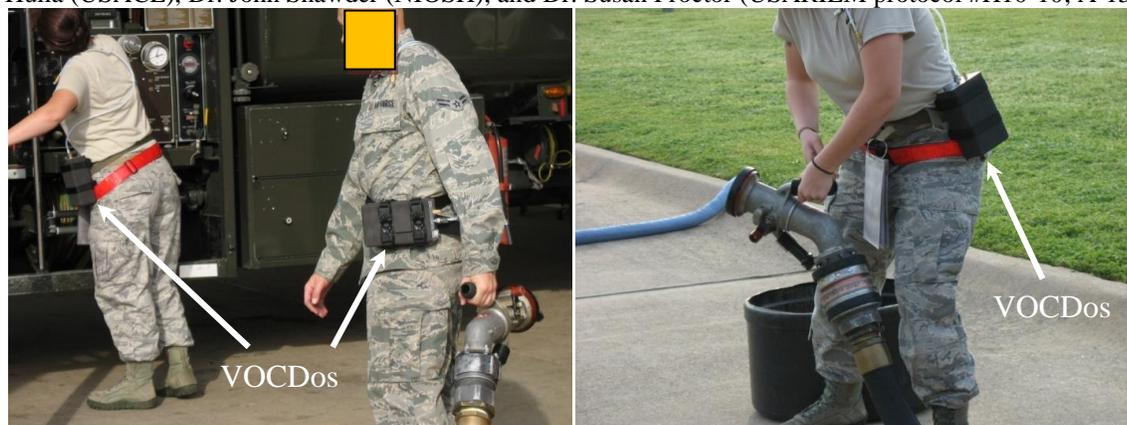
Figure 9. Photos of VOCDos personal exposure monitor during JetA fueling operations
