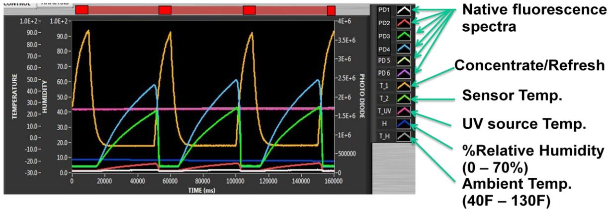
Figure 5. Illustration of cyclic operation of VOCDoS sensor. Shown for 4 measurement cycles, time shown in milliseconds.
